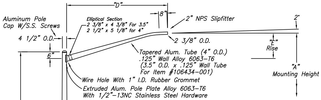
This Pole Has Been Designed For 90 MPH Wind Speeds (3 Second Gust) Per AASHTO LTS-6 (2013) And All Interim Revisions When Supporting One Fixture With An EPA = 1.5 Sq. Ft. And Weighs 30 Lbs.
